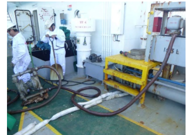
Wilden pump at F.O no. 3 vent
